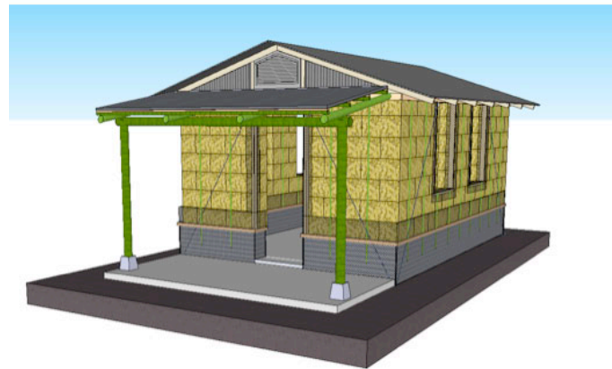
The Ti Kay Pay unplastered, showing mesh over gravel bags, bamboo stiffeners over straw bales, and diagonal wire bracing
