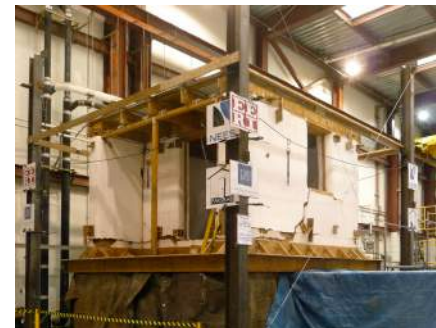
Shake-table test of Pakistan straw bale wall system in 2009 at the Univ. of Nevada, USA.
